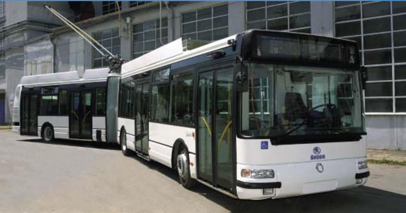
SKODA 25Tr IRISBUS is a new high-capacity low-floor trolleybus using the advantages of progressive electrical equipment SKODA and a body of an 18-metre articulated bus AGORA City Bus from the production of the IRISBUS Group.
